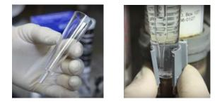
A continuous flow of sample through the tube prevents contamination from atmospheric oxygen. When the operator submerges the vacuum-sealed ampoule in the flowing sample and snaps the tip, sample is drawn into the ampoule. The highly sensitive colorimetric Rhodazine D<sup>TM</sup> reagent reacts instantaneously to produce a pink color.
