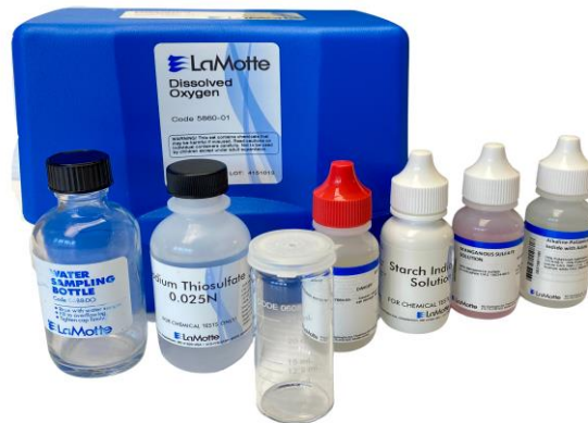
The LaMotte 5860-01 test kit utilizes the Winkler method for Dissolved Oxygen analysis.
