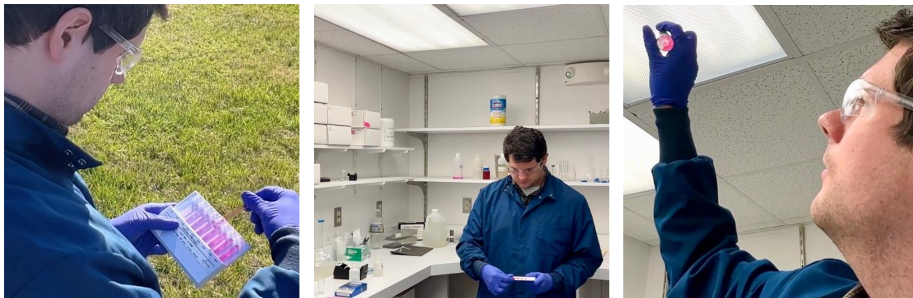
Figure 1: Comparators can be read under various light sources including outdoors, fluorescent light, and LED light.
