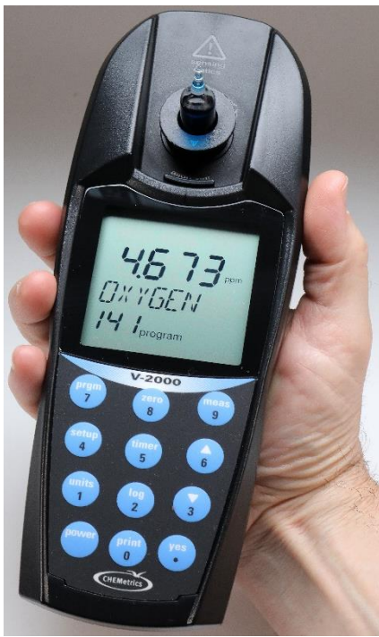
Figure 2: A V-2000 can read multiple CHEMetrics tests including COD.
