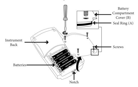
To ensure that the instrument is waterproof:
