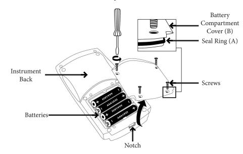
To ensure that the instrument is waterproof:
