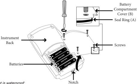
To ensure that the instrument is waterproof:
