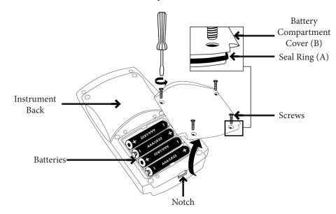
To ensure that the instrument is waterproof:
